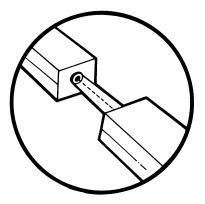
Any potentially dangerous laser beams must be enclosed or otherwise made inaccessible to visitors. The enclosures or guards must be sturdy enough and well enough secured to resist normal bumps and jostling and even casual, curious removal. An example, using simple materials, is shown here. A clear plastic tube encloses a laser beam as it passes from one device to another; the tube is firmly attached to each device. **Demonstrating Internal Laser Elements**
