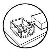
A simple, but sturdy, plastic box can be used to enclose tabletop space in which multiple beams are involved in various interactions. Once again, carefully check to see that no stray beams leave the box; block them internally. This technique has the additional advantage of preventing curious visitors from readjusting the alignment.
