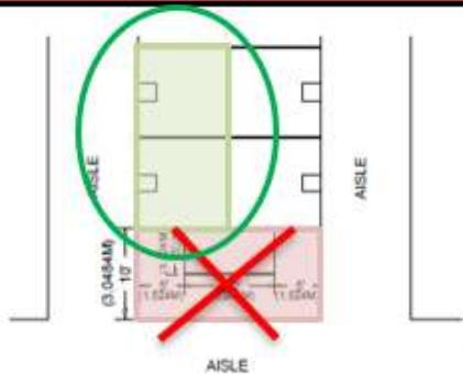
Island Booths: Island booths are exposed to aisles on all four sides. There is no pipe and drape construction provided.
