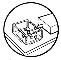
A simple, but sturdy, plastic box can be used to enclose tabletop space in which multiple beams are involved in various interactions. Once again, carefully check to see that no stray beams leave the box; block them internally. This technique has the additional advantage of preventing curious visitors from readjusting the alignment.
