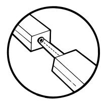
Any potentially dangerous laser beams must be enclosed or otherwise made inaccessible to visitors. The enclosures or guards must be sturdy enough and well enough secured to resist normal bumps and jostling and even casual, curious removal. An example, using simple materials, is shown here. A clear plastic tube encloses a laser beam as it passes from one device to another; the tube is firmly attached to each device.
