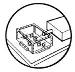
A simple, but sturdy, plastic box can be used to enclose tabletop space in which multiple beams are involved in various interactions. Once again, carefully check to see that no stray beams leave the box; block them internally. This technique has the additional advantage of preventing curious visitors from readjusting the alignment.
