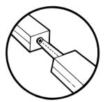
Any potentially dangerous laser beams must be enclosed or otherwise made inaccessible to visitors. The enclosures or guards must be sturdy enough and well enough secured to resist normal bumps and jostling and even casual, curious removal. An example, using simple materials, is shown here. A clear plastic tube encloses a laser beam as it passes from one device to another; the tube is firmly attached to each device.
